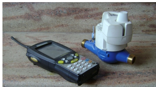
Hand held unit and water meter equipped with AMR technology
