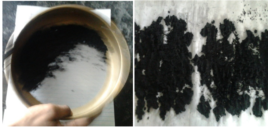
Fig 1 Burning, Crushing, Sieving, Washing and Drying of AC
