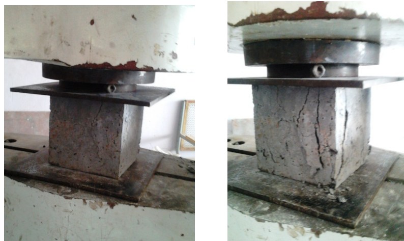
Fig 9 Compression test on the replaced concrete
