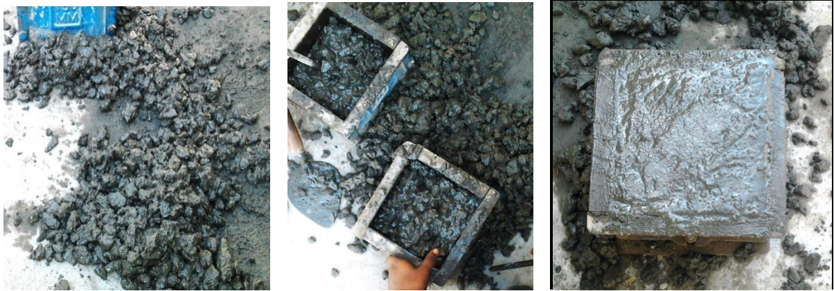
Fig 8 Casting process of the replaced concrete
