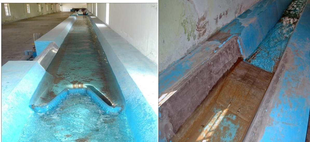
Figure 3 and 4. : Long-throated flume and Long-crested weir in CWPRS model canal
