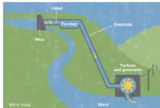
Fig 3: Run Off River Scheme
