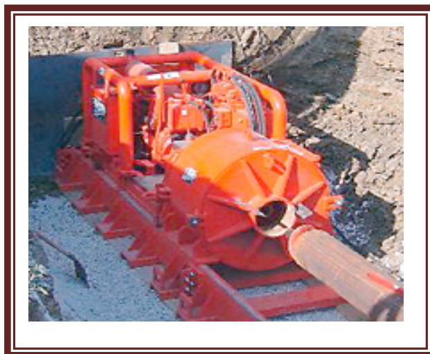
Auger Boring Machine
