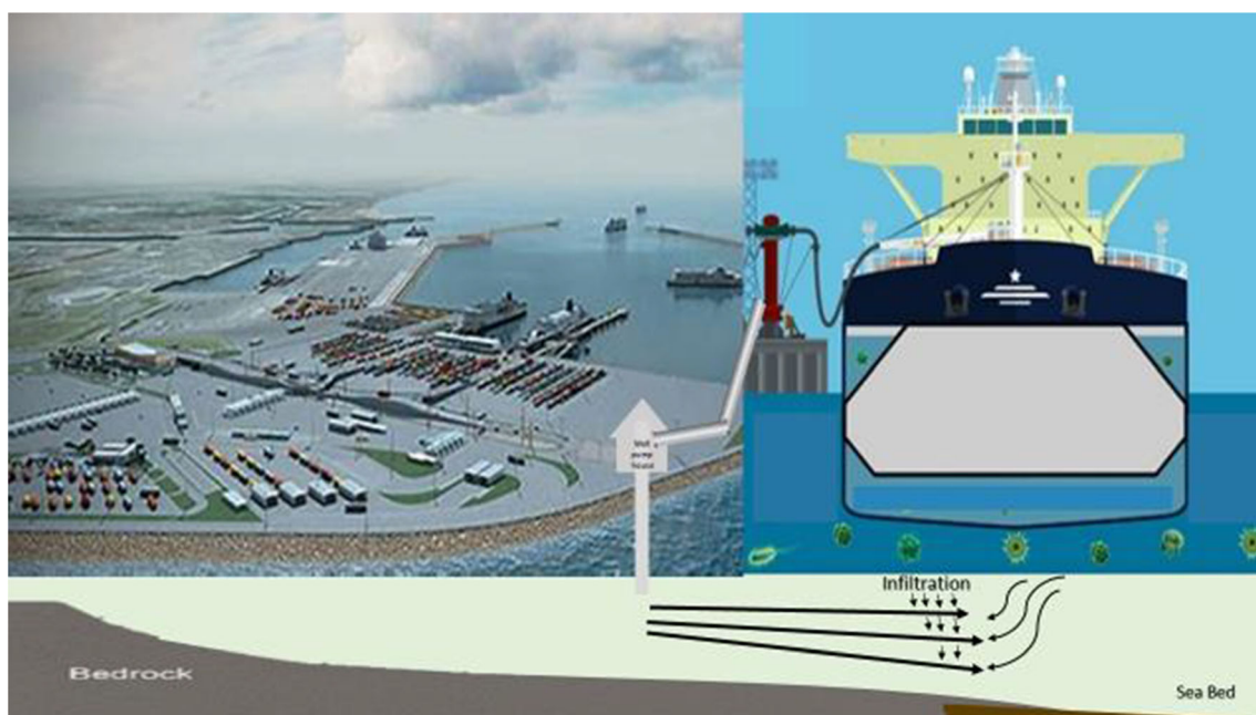
Fig. 3 Schematic diagram of the use of well filtration systems on seabed infiltration galleries to supply ship ballast water. Note that pipelines and storage tanks would be installed adjacent to the docking facilities
